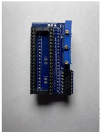
Attention: After adding this fix, if you have removed your stock heatsink for the VIC-II chip you MUST add some heatsinks to it. It WILL get hot and will overheat and shut down quickly.
