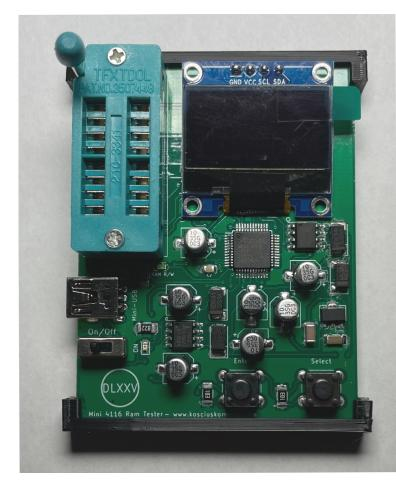
At the top is the ZIF 16 pin socket and the OLED display. Under the ZIF socket there is a female mini-usb socket. This is used to power the unit. It requires 5V so you can use any usb power source that is 5V. Below the usb port if an on/off switch. This allows you to turn the unit off and on while leaving it plugged into the power source.
